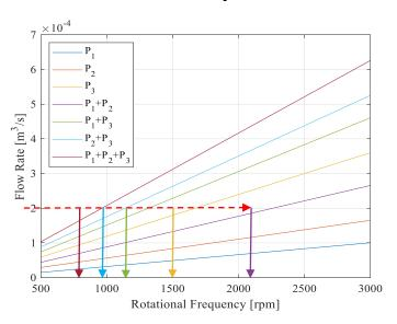
Different pump unit combinations for a same flow rate
