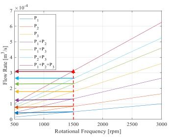
One flow rate for each pump unit combination
