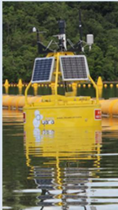
Buoy to survey water quality parameters in hydroelectric dams
