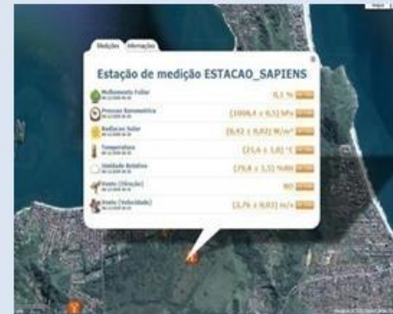
Sensor network to survey environmental parameters in a science and technology park
